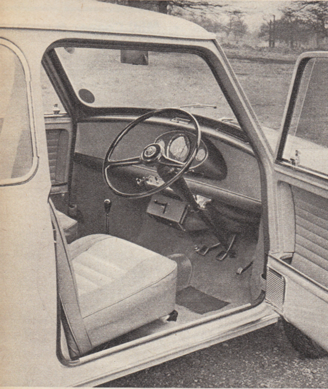
A familiar Mini-Cooper interior but for the revised fresh air heater with fan, mounted centrally beneath the parcel shelf
